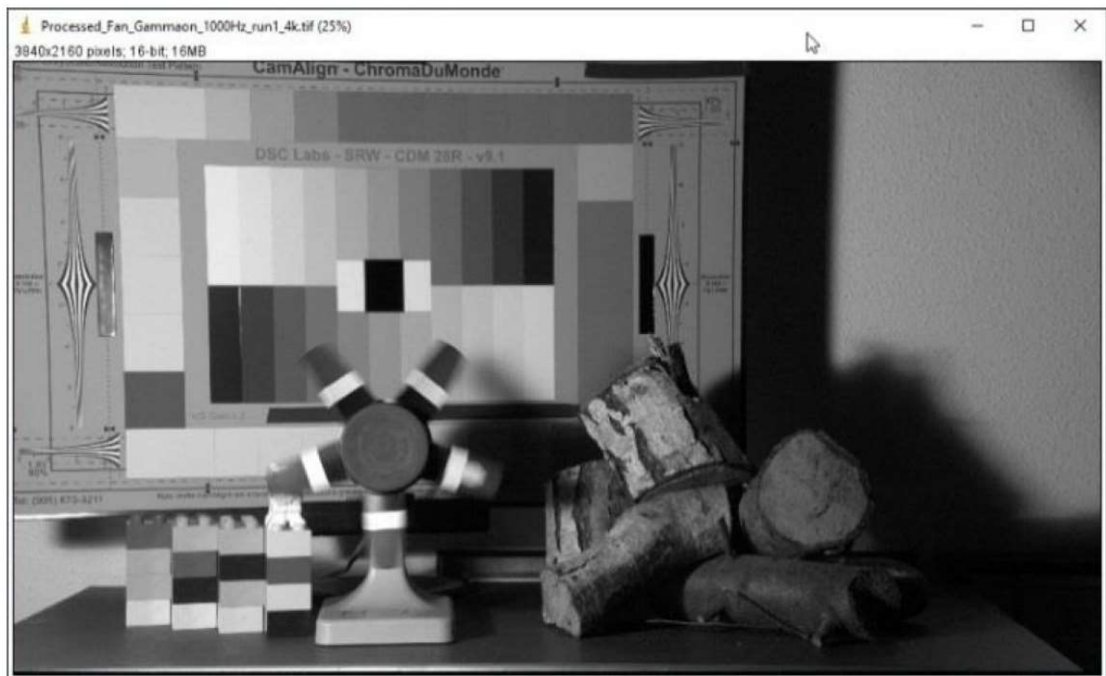
Figure 5 - Sample UHD image at 60 fps with integration time of 1ms
