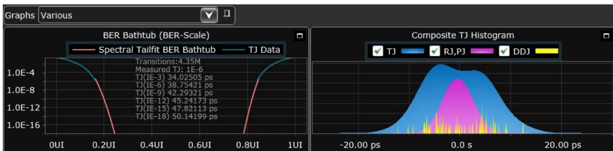
Figure 7 - Serializer BER bathtub and total jitter histogram
